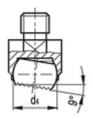
$$\begin{array}{lll} d1 & = 13 \\ d2 & = M8 \\ d3 & = 7.2 \\ d4 & = 10 \\ l1 +/-0.1 & = 13 \\ l2 & = 8 \\ Max \ static \ load \ (KN) = 10 \\ \end{array}$$
